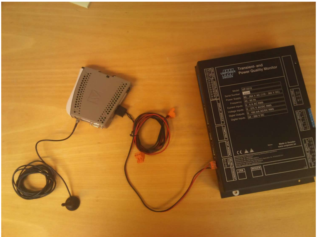
Figure 47 - GDW-11 GSM/GPRS modem with RS-485 connection to a meter
